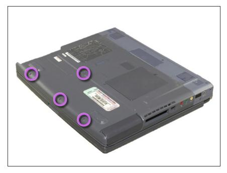
Remove the four 16 mm screws bordering the edge of the laptop using a Phillips #0 screwdriver.
