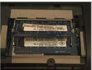
Gently pull apart on these metal tabs and the RAM will pop up. This can then be safely removed by hand.
