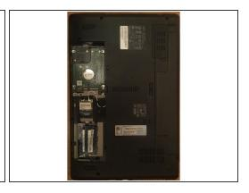
Using an opening device; insert it into the notch, and slide the device along all sides to pop the plate out.
