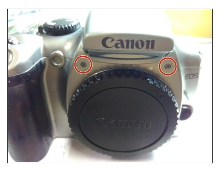
Remove the two 7mm philips screws from the front casing.
