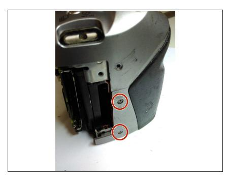
Remove the two 1/8" philip screws from the right side of the front casing.
