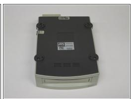
Pry all four of the plastic feet off the bottom of the enclosure using the iPod opening tool.
