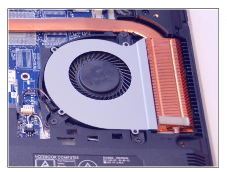
Gently lift the fan out of its slot.
