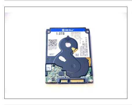
Remove the HDD from its location.
