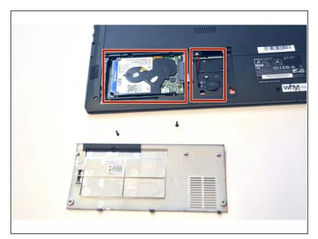
HDD hard disk and BIOS stack components appear.
