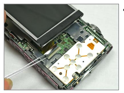
• Use the <u>tweezers</u> to lift the ZIF connector which is holding the ribbon cables that connect the LCD screen to the motherboard.
