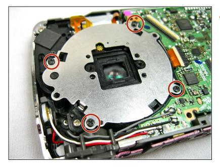
Remove four 3.4 mm black screws from around the perimeter of the silver plate.
