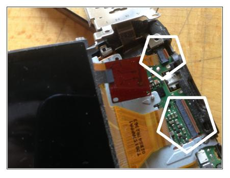
The display is plugged in the camera with 3 little connectors. Carefully click the hinge open and you can pull out the connector.
