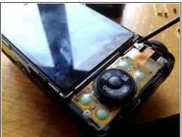
You only need one small cross screw head screwdriver to open up the camera. It takes 9 screws to take out the display.
