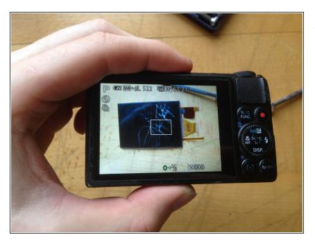
replace the display, plugin the connectors, and screw it back together. It should work again right after you turn it on
