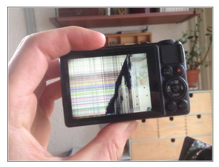
So that's the problem: a cracked screen. The rest still works fine.
