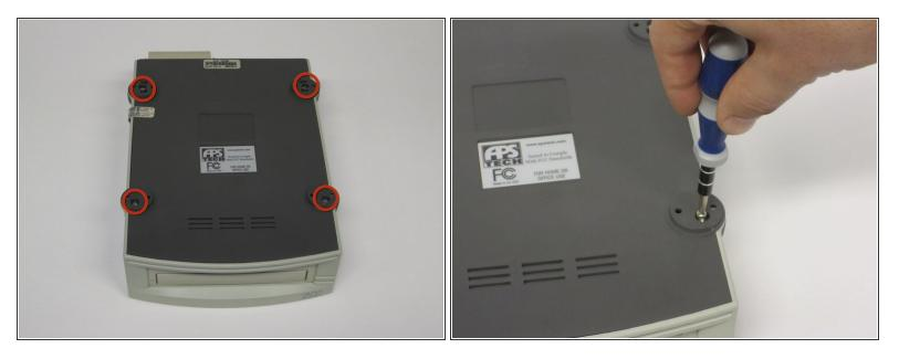
Unscrew the four screws previously covered by the feet with a Phillips #1 screwdriver.
