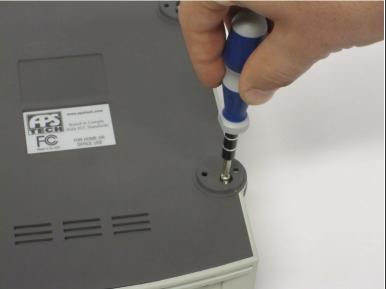
• Unscrew the four screws previously covered by the feet with a Phillips #1 screwdriver.
