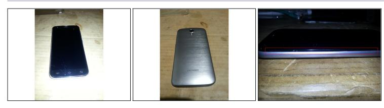
• Start by flipping the phone over and removing the back plate by applying a small amount of of prying, between the glass screen and the plastic back, indicated in red in the picture. If having trouble I recommend a plastic prying tool.
