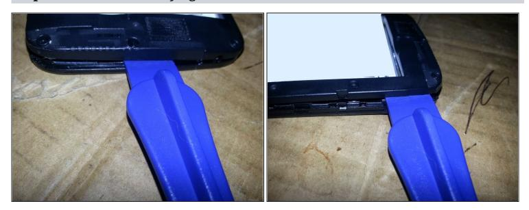
• Using a plastic prying tool to carefully separate the back plastic cover (first mid frame) from the second mid frame. I recommend starting at the bottom and slowly work your prying tool around from there.
