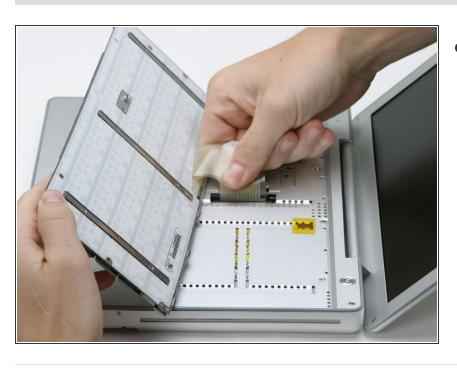
Grasp the keyboard connector ribbon near the connector and disconnect it from the logic board.
