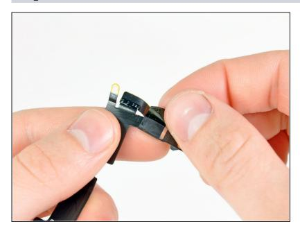
Carefully remove the strip of tape covering the front camera cable connector.
