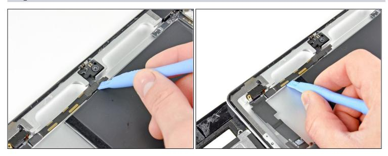
• Use the edge of a plastic opening tool to peel the tape and the adhesive securing the headphone jack & front camera cables to the rear panel.
