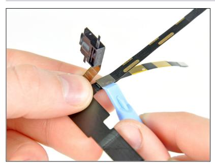
Use the edge of a plastic opening tool to disconnect the front camera cable from the headphone jack cable.
