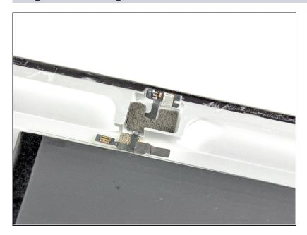
Peel the piece of foam up off the top of the microphone cable assembly.
