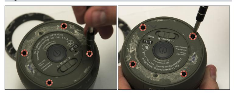
• Use a Phillips #1 screwdriver to remove the four black 9mm screws from the device.
