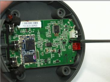
• Remove the three black 6mm screws from the main board using a Philips #00 screwdriver.
