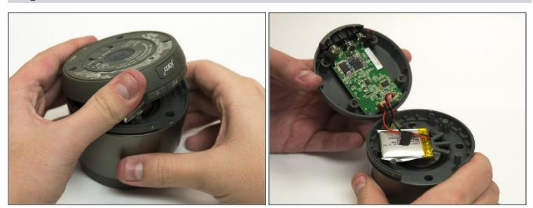
Gently separate the base from the rest of the device to reveal the battery and the main board.
