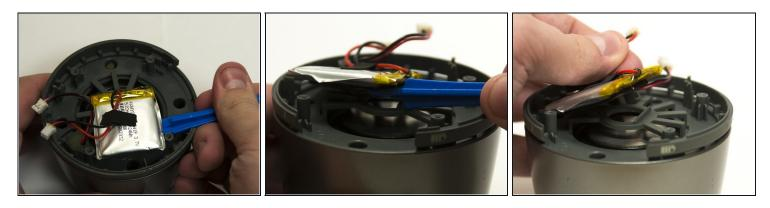
⚠ Batteries can be very dangerous if punctured. Use extra caution when using tools around the battery.
