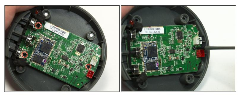
• Remove the three black 6mm screws from the main board using a Philips #00 screwdriver.
