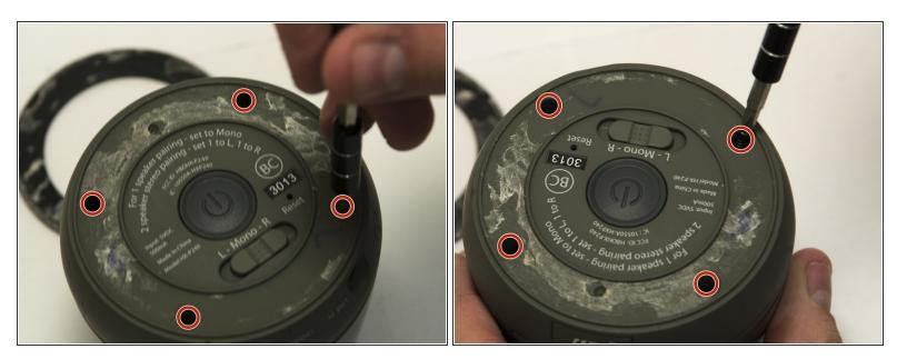
Use a Phillips #1 screwdriver to remove the four black 9mm screws from the device.
