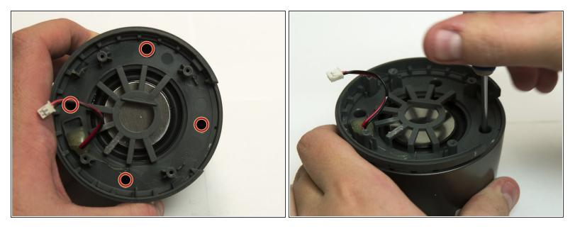
• Use a Phillips #1 screwdriver to remove the four black 9mm screws from device.
