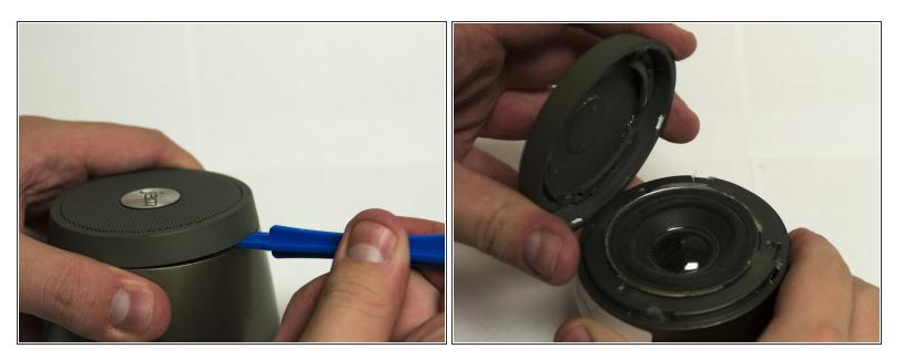
• Use the plastic opening tool to separate the speaker grate from the rest of the device.
