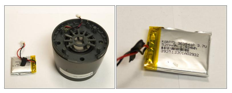
Solution Use new adhesive to secure battery back to the rest of the device.
