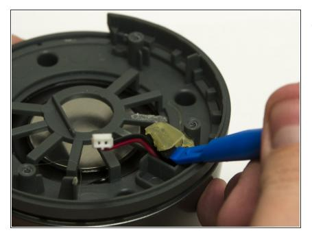
Use the plastic opening tool to pry the glue away from the wire. Be careful not to damage the wire.
