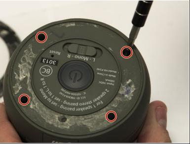
• Use a Phillips #1 screwdriver to remove the four black 9mm screws from the device.
