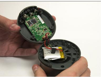
Gently separate the base from the rest of the device to reveal the battery and the main board.
