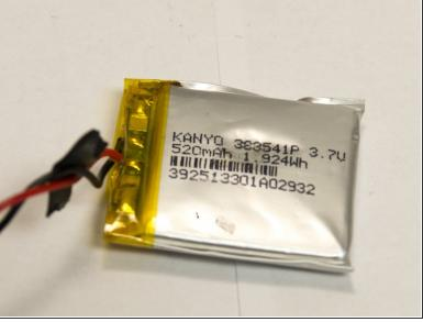
Use new adhesive to secure battery back to the rest of the device.
