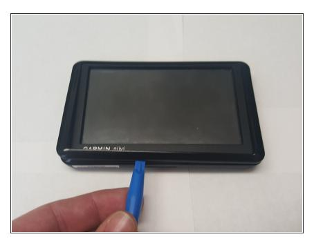
Snap the plastic cover off using a plastic opening tool.
