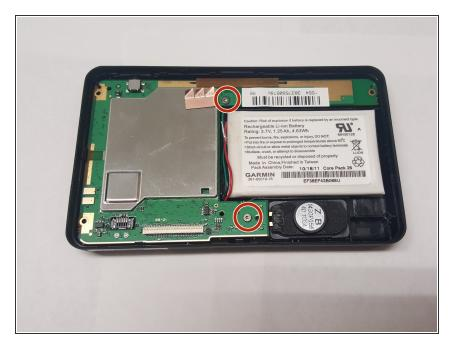
Remove the two silver 5 mm T5 torx screws connecting the circuit board to the plastic casing.
