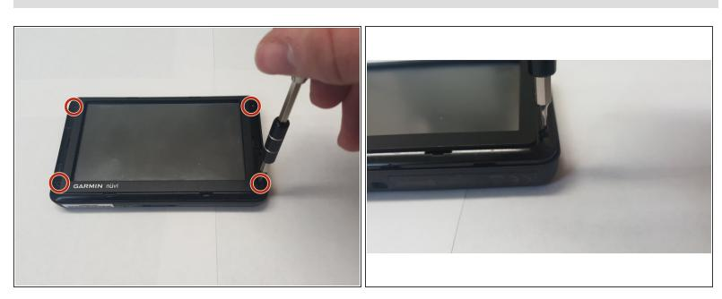
Remove the four black 11 mm T5 torx screws.
