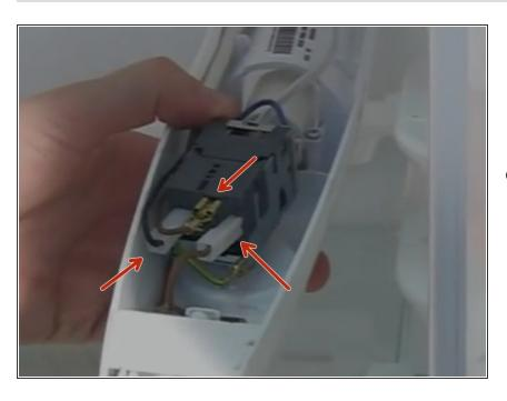
Remove the three cords on the front side of the thermostat by simply pulling the plastic connector off for two connections and doing the same for the metal connection. Do the same to the back side, disconnecting another plastic connector and then remove the thermostat.
