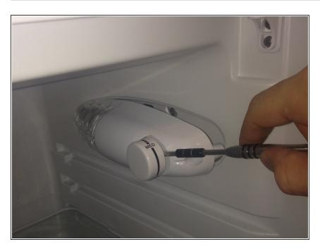
Carefully remove the thermostat knob.
