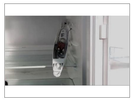
Once the thermostat is removed, take a picture of the cords (still connected) to help with reassembly.
