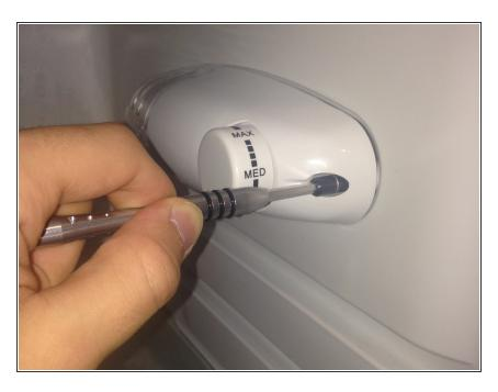
Remove the 28 mm screw holding the thermostat to the refrigerator using the JIS #1 screwdriver
