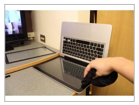
Finally, use the screen cleaning cloth and carefully press the edges of the screen one more time.
