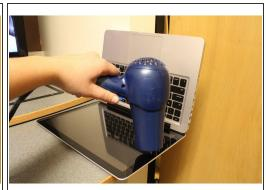
To insure the seal of the adhesive, reheat it again with the hair drying.
