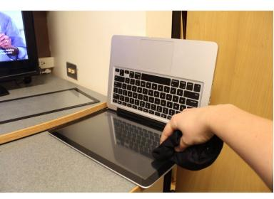
Using the screen cleaning cloth carefully press the edges of the screen to seal the adhesive.
