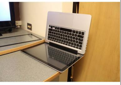
Place the new screen in position. Confirm that the new screen is properly aligned with the edges of the Macbook Pro.
