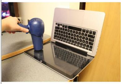
• Use a hair dryer to heat the adhesive around the edges of the screen you are removing.
