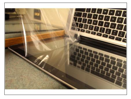
Peel the protective covering off the new screen.
