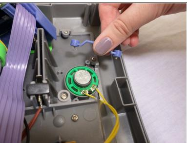
• Using the ifixit screwdriver with phillips head J1, unscrew the two screws located on the ends of the purple piece covering the speaker. Place screws onto Magnetic Mat.
