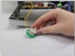
Place the sticky side of the felt pad directly in the center of the clear plastic covering on speaker.
