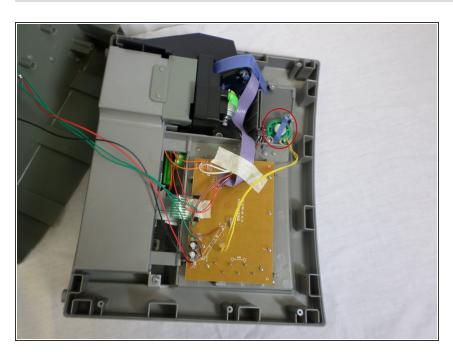
The Zillionz ATM Machine Speaker is placed on the upper left of the machine. The speaker is a circular green shape with a thin purple cover holding the speaker in place. There will be two yellow wires connecting the speaker to the circuit board.
