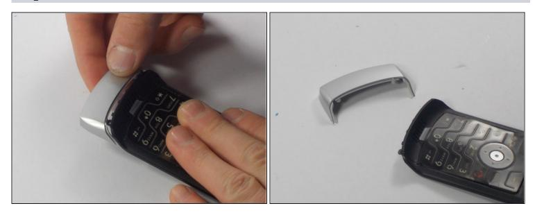
• Remove the keypad cover, located below the keypad on the front of the phone.
