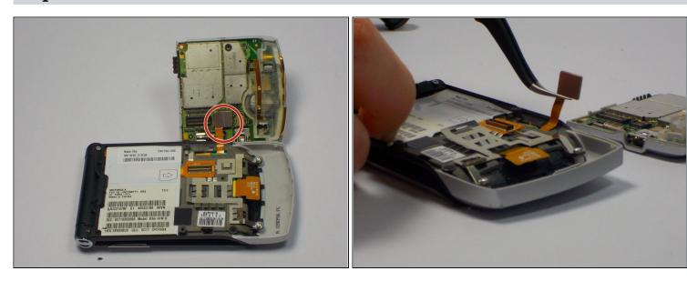
• Use <u>tweezers</u> to disconnect the copper ribbon from the inside of the back panel.
