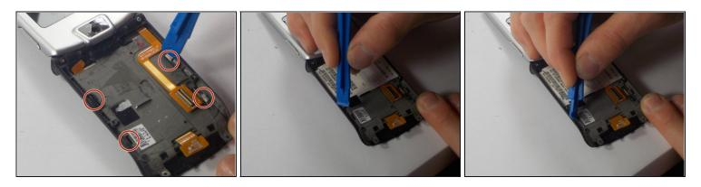
Using a plastic opening tool, push the four metal tabs along the edge of the phone in towards the keypad.
