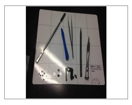
Tools necessary for task. Starting from the left to right Metal Spudyer Plastic opening tool Precision tweezer Point pen tool Driver with bit size J0
