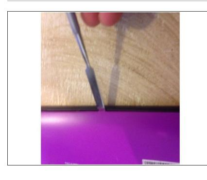
The backing of the tablet is fastened by simply snapping it in. Using the metal opening tool, pry between the plastic backing and the edge, but do not remove it yet. Work your way around until you have them separated.
