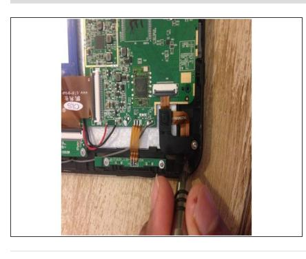
You can directly locate and remove the camera component in the corner. Simply unscrew the piece and gently remove the tape wire.
