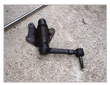
First the Idler arm must be removed from the truck. Another guide has instructions to take the arm off.
