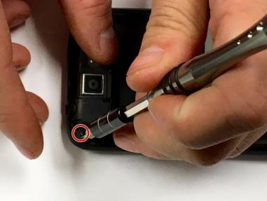
Take out the upper, two 0.5 mm Torx screws with a Torx T5 bit.
