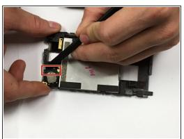
Using the spudger, pry the speaker out of its place.
