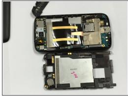
Using the spudger, pry up to remove the battery holder.
