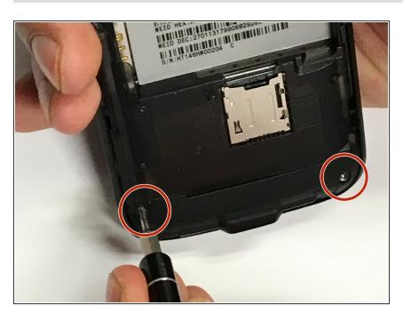
Remove the lower, two 0.5 mm screws using Torx T5 screwdriver.
