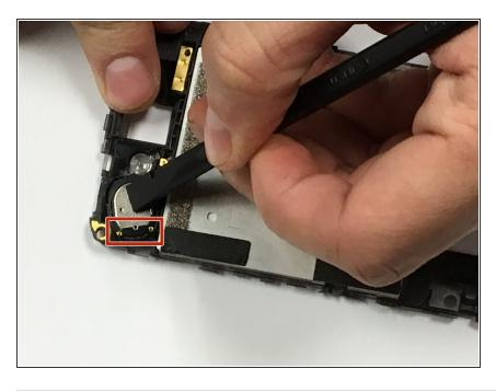
With the springs up, place the new speaker into position.
