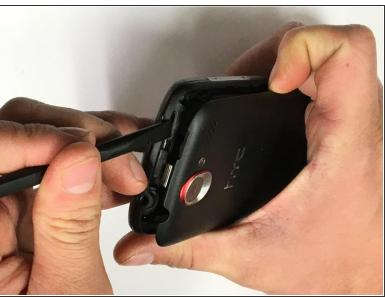
Insert flat end of spudger into slot on the top of phone to pry off the back plate.
