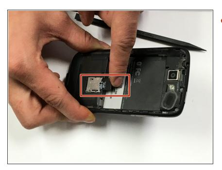
Remove SD card and replace with a new one.
