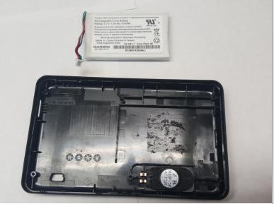
Peel the battery from the plastic back with a plastic opening tool.
