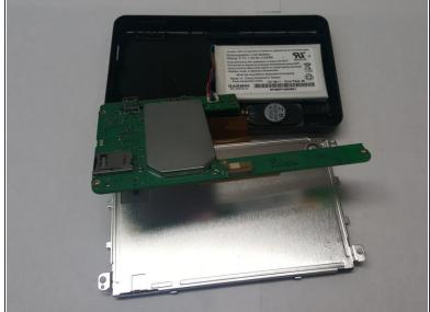
Flip the circuit board over onto the screen.
