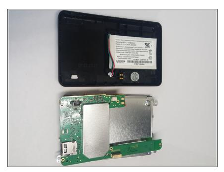
Disconnect the harness between the battery and the circuit board.
