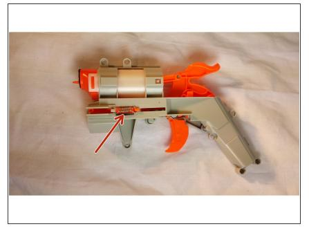
• Remove the exterior spring from the sliding mechanism and re-position the gun on its opposite side.
