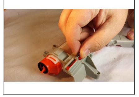
Reconnect the spring to the orange slider, and connect the orange slider to the grey hook.
