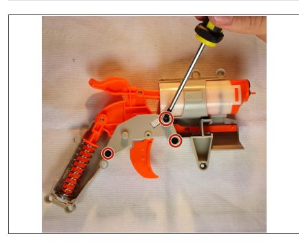
• Remove the three screws holding the trigger plate in place, then remove the plate carefully.
