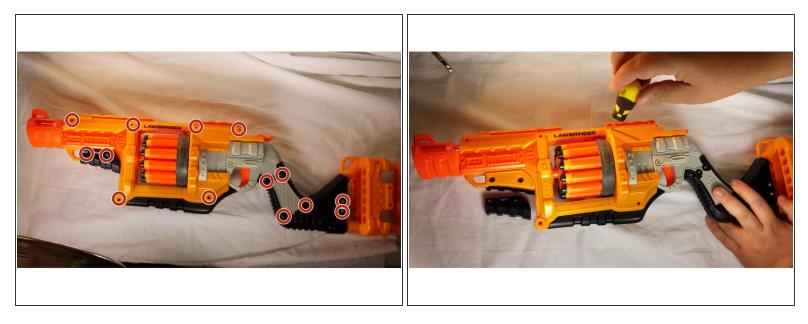
• Locate and remove all 14 screws of the outer case and gently remove it avoiding any damage.
