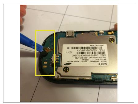
Use the plastic opening tool to pry the logic board out of the phone case from the bottom area of the phone.
