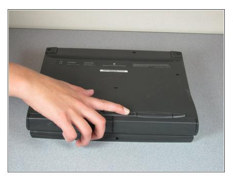
Slide the latch to the left to release the battery.
