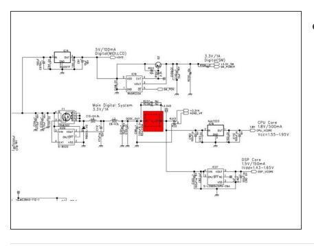
Here is the fuse marked red in the EMX Service Manual from Korg. The part we are dealing with seems to be identical with the ESX
