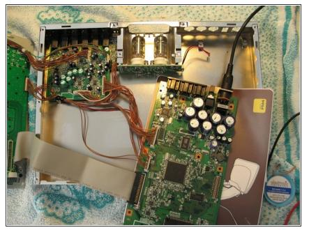
Unplug all cables and the power supply. Remove all Knobs by pulling on them. Then unscrew all screws on the front using an allen key. You can remove the PCBs as well, as shown on the picture, but you don't have to.
