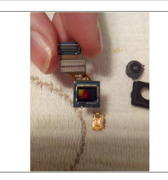
We must now separate the blue film and casing from the camera's sensor. This is done by wedging an x-acto knife in between the sensor board and the casing.
