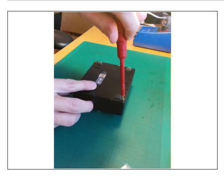
Open the back of the case by undoing the 4 screws with a regular philips screwdriver.
