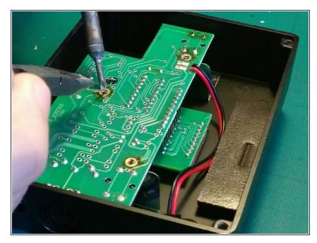
Fit the board to the mount points and apply generous solder. Make sure to check that the display fits and it's correctly aligned with the case before soldering.
