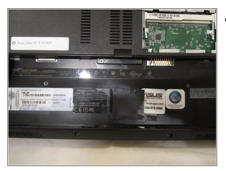
Remove the four 3mm screws from underneath the battery.
