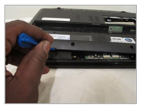
• Use a plastic opening tool to pry the case open and remove it.
