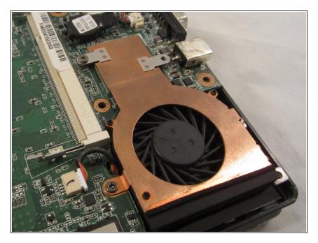
• Locate the fan and remove the screws (3mm).
