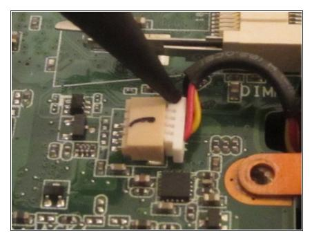
• Use a spudger to remove the power supply.
