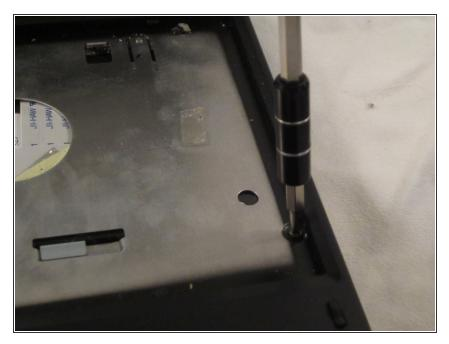
• Remove the screws from under the keyboard. (Two 7mm and five 5mm)
