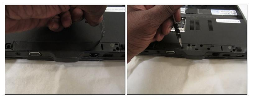
• Peel the black strip off of the back of your Asus Eee PC T101MT to expose more screws. Remove screws from the outside of the device case (ten 7mm screws and two 8mm screws).
