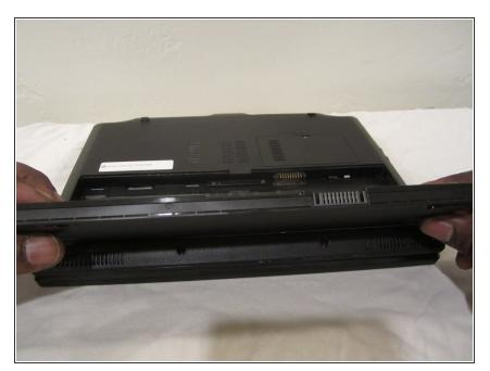
• Lift the battery out of the device.
