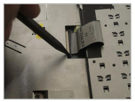
Once you have the keyboard out, use the nylon spudger to remove the connection. You can now replace the keyboard.
