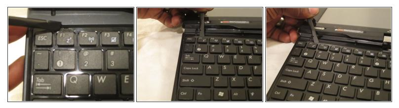
• Turn the tablet over and open it up. Insert a nylon spudger into the slots above F1, F6, F10 to pry up the keyboard.
