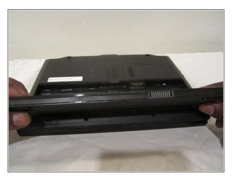
Lift the battery out of the device.
