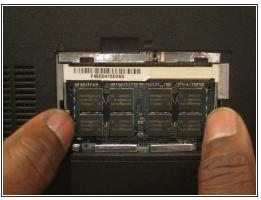
In order to release the RAM module, you will need to move the metal tabs on both sides at the same time. This can be accomplished by using plastic opening tools or your fingers.
