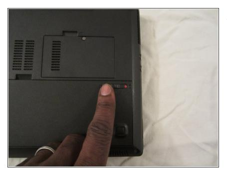
Locate the sliding tab on the right and slide it to the left in order to unlock the battery.
