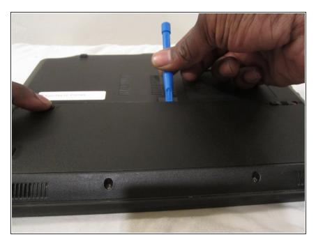
Use a plastic opening tool to lift the battery up as you slide the tab on the left to the right.
