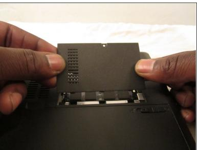
Use a plastic opening tool to remove the cover.
