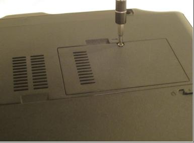
Grab a drive adapter and a PH0 phillips head bit and use the screwdriver to remove the 5mm screw from the cover of the compartment.
