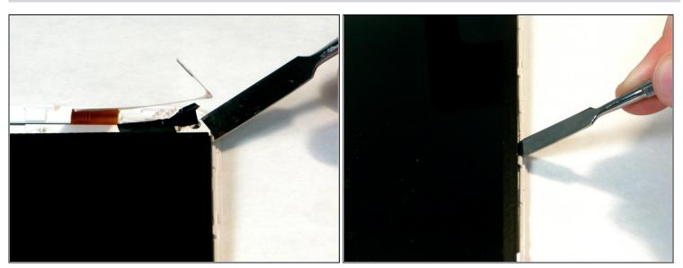
• Start in the top right corner of the tablet and use a spudger to work your way down the right side, further separating the screen and the tablet.
