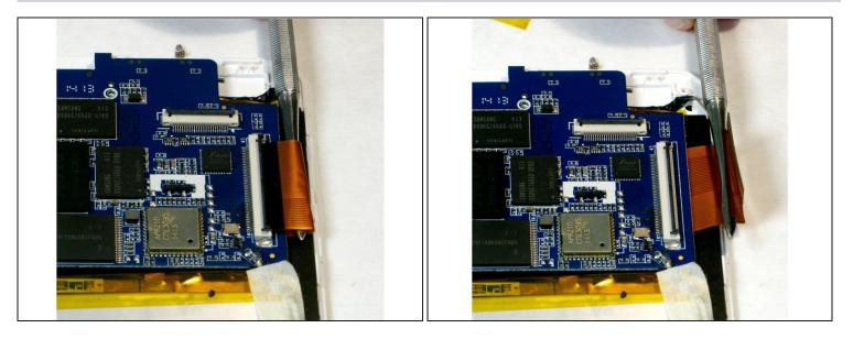
• Use a spudger to lift the right side of the ribbon cable and disconnect it from the motherboard.
