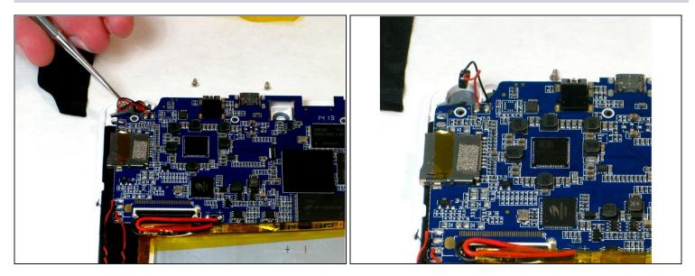
• Locate the microphone in the top left corner of the tablet. This piece easily pops our of the hole it is sitting in with the help of a spudger.
