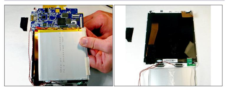
• After all of these steps, the motherboard, speakers, and battery should all be able to be removed as one piece. The battery may have adhesive retaining it. To remove it work a pry tool underneath carefully separating it from the back of LCD screen.
