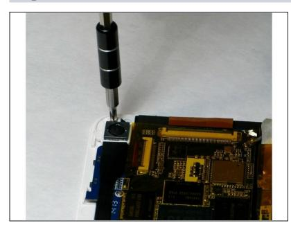
• Take the Phillips head screwdriver and unscrew the 3mm screw right above the camera assembly. Place the screw aside so you do not lose it.
