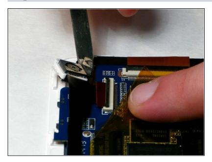
Now you can remove the camera assembly. Use a spudger to gently loosen the camera out of place.
