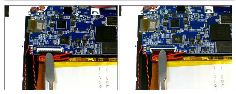
• Find the second ribbon cable near the top left corner of the tablet.
