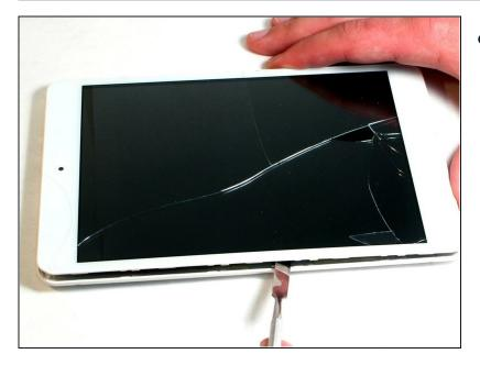
Starting near the middle edge of the Trio Stealth-G4X tablet, gently work an opening pick or spudger in between the seams of one side of the tablet.
