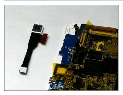
• You have now removed the camera assembly and can set it aside. Insert replacement camera by following the steps in reverse. Then reassemble the tablet the same way.
