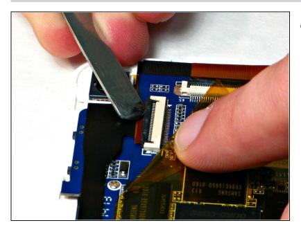
• Peel back the yellow protective film on the motherboard to access the camera's ribbon cable.
