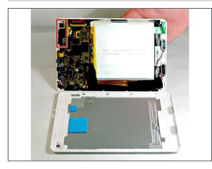
Once the two halves are separated, set aside the back cover of the tablet as you will not need it until reassembly. Now locate the camera on the motherboard of the tablet.
