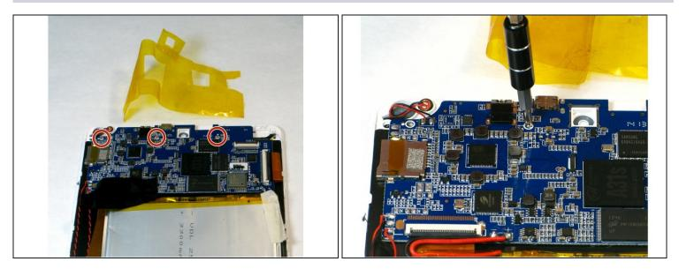
• Remove the three remaining 3 mm screws from the motherboard using a Phillips screwdriver.
