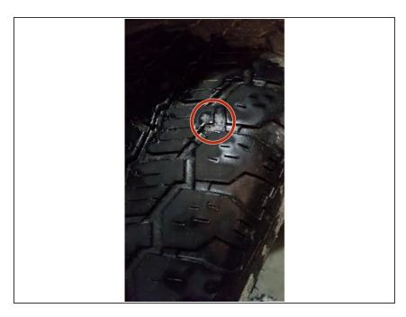
Look for tiny air bubbles forming from the leaking air and soap combination, this is where the hole is located.
