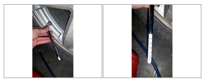
• Use the air pressure gauge to make sure the tire is now aired up to its original pressure.
