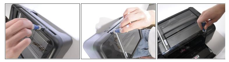
• Remove the three screws from the top of the printer with a T-9 screwdriver as shown.
