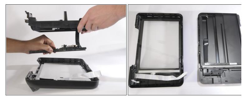
A Carefully separate the two hood pieces connected by the black ribbon.
