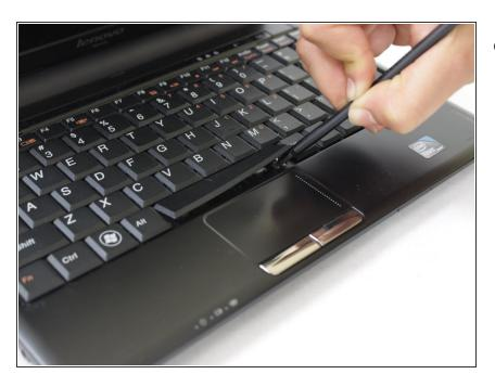
Use a spudger to remove the keys by wedging it underneath the key.
