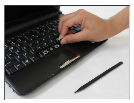
Pull back the key to remove and separate the key from the metal bars underneath.
