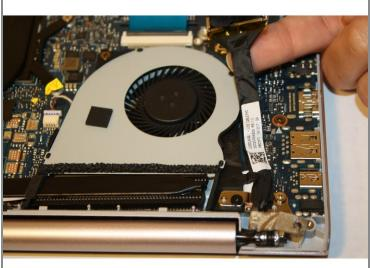
• Remove the LVDS cable next to the cooling fan.
