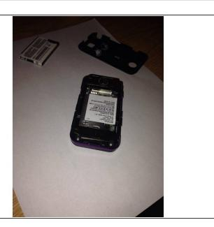
Place index finger an thumb on the battery and pull away from device.
