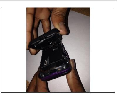
Push down on the lever, while pulling the back cover away from the device
