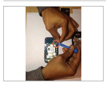
Using the pry tool, remove the lock/mute button.
