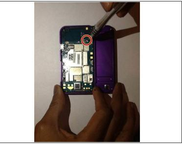
Using a screw driver, locate and remove the screws that connect the keyboard to the mother board.
