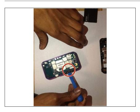
Using the pry, remove the volume buttons.
