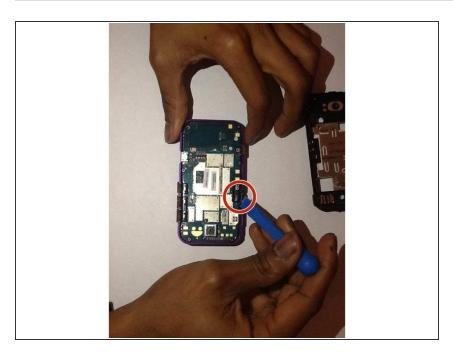
Using the pry tool remove the camera button from the phone.
