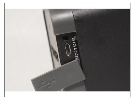
Make sure there is no unwanted debris located in the USB charging port and the hole that holds the protector in place.
