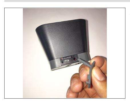
Align the port protector with the port protecting hole that keeps the plastic covering in place.
