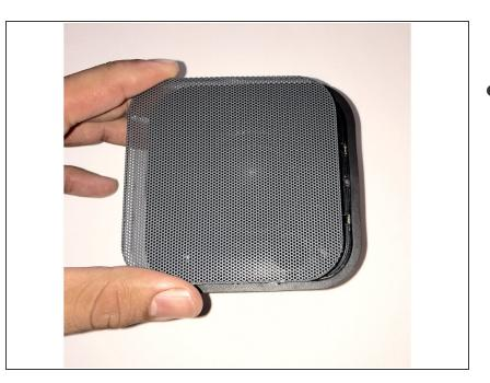
Line up the replacement metal covering with the interior square ridge of the speaker.
