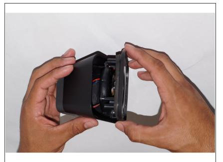
With the screws removed, you can now remove the top piece of the speaker to gain access to the interior.
