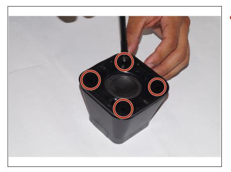
You can now use the Phillips #00 screwdriver to remove the four screws.
