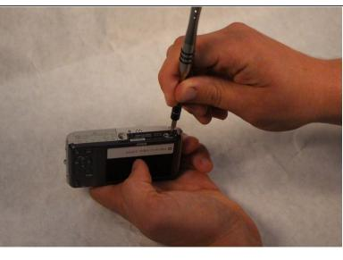
With the battery door facing upward, take your PH000 screwdriver and remove the 4 mm screws from the bottom of the device.
