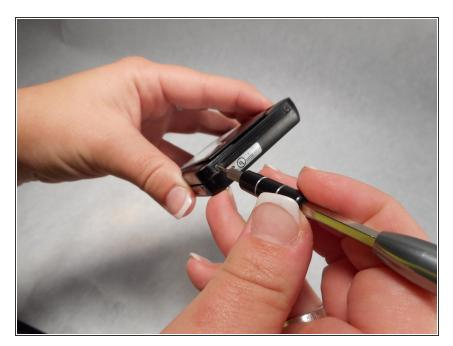
Using your Phillips #00 screwdriver, remove all four 0.3 cm screws that are located on both ends, as well as the bottom of your Cyber-Shot
