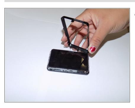
The back case of the device is the metal frame.
