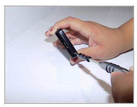
Using the Phillips #00 Screwdriver, remove all of the 0.3 cm screws from both left and right panels.
